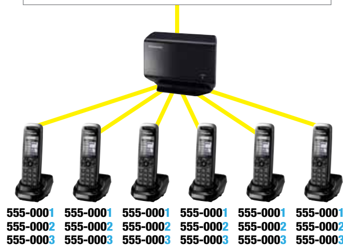
6 Station: 3 Line "Key" System
